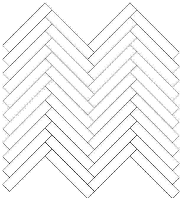
\*\*Laying tiles with maximum 1/4 shifting from the long edge of the rectangular tiles is recommended. Laying tiles with 1/2 shifting from the tiles is not recommended.
